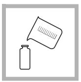
**6.** Fill a second sample cell with 10 mL of sample (the blank). Place it into the cell holder.
