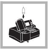
**10.** Within 3 minutes after the timer beeps, place the AccuVac Ampul into the cell holder. Close the light shield. Result in mg/L iodine will be displayed.
