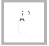
**4.** Add the contents of one DPD Total Chlorine Powder Pillow to the sample cell (the prepared sample). Swirl to mix.
