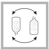
**6.** Quickly invert the ampul several times to mix. Wipe off any liquid or fingerprints.
