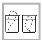
**5.** Fill a DPD Total Chlorine Reagent AccuVac Ampul with sample.
