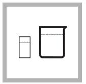
**4.** Fill a zeroing vial (the blank) with at least 10 mL of sample. Collect at least 40 mL of sample in a 50-mL beaker.
