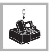
**8.** Place the blank into the cell holder. Close the light shield.
