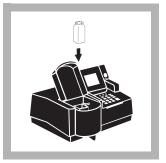
**8.** Within 3 minutes after the timer beeps, place the prepared sample into the cell holder. Close the light shield. Result in mg/L I<sub>2</sub> (or chosen units) will be displayed.
