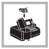
**3.** Insert the AccuVac Ampul Adapter by sliding it under the thumb screw and into the alignment grooves. Fasten with the thumb screw.
