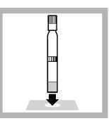
**13.** Remove the blank value cuvette.
