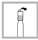
**5.** Blank value cuvette preparation: Carefully remove the foil from the screwed-on **DosiCap Zip**.
