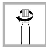
9. Immediately screw the **DosiCap Zip**, with the fluting at the top, back onto each cuvette.
