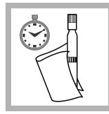
**11.** After **3 minutes**, thoroughly clean the outside of the cuvettes and evaluate.
