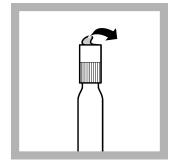
1. Sample cuvette preparation: Carefully remove the foil from the screwed-on **DosiCap Zip**.
