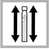
Immediately put the cap on the vial. Hold the vial by the cap, over a sink. Shake the vial quickly. The vial gets very hot during mixing.
