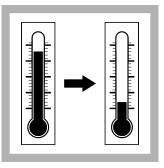
8. When the timer expires, set the reactor power to off. Let the temperature decrease for about 20 minutes to 120 °C (248 °F) or less.
