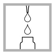
**2.** Use a pipet to add 1.8 mL of sample to the test vial.
