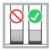
**12.** Wait for the sediment to fully settled to the bottom of the vial. If necessary, put the vial in a centrifuge at 4000 rotations/minute.
