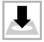
**14.** Insert the vial into the cell holder. DR1900 only: Push **READ**. Results show in mg/L COD.
