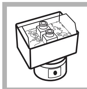
5. Pipet 0.5 mL of the filtrate or supernatant into another dry 25-mL sample cell (the prepared sample).
