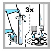
**6.** Rinse the sample vial and cap three times with the sample.
