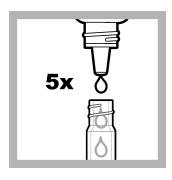
9. Immediately add 5 drops of Fluorescence Sulfite Reagent 2. Hold the bottle vertically.
