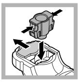
**3.** After startup, install the vial adapter. Push in the tabs on the sides of the vial adapter as shown.
