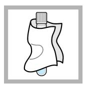
**13.** When the timer ends, clean the external surface of the sample vial with a no-lint cloth.
