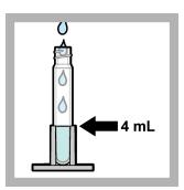
7. Put the sample vial in the sample vial holder. Add the sample to the top of the sample vial holder (4 mL).
