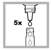
8. Immediately add 5 drops of Fluorescence Sulfite Reagent 1. Hold the bottle vertically.
