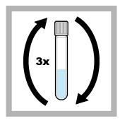
**10.** Put the cap on the vial. Invert the vial 3 times to mix. Put the vial in the sample vial holder.
