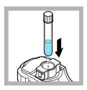
**14.** Put the sample vial in the vial adapter.
