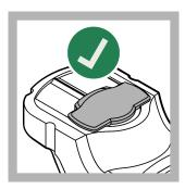
**2.** Keep the sample port cover closed during startup.
