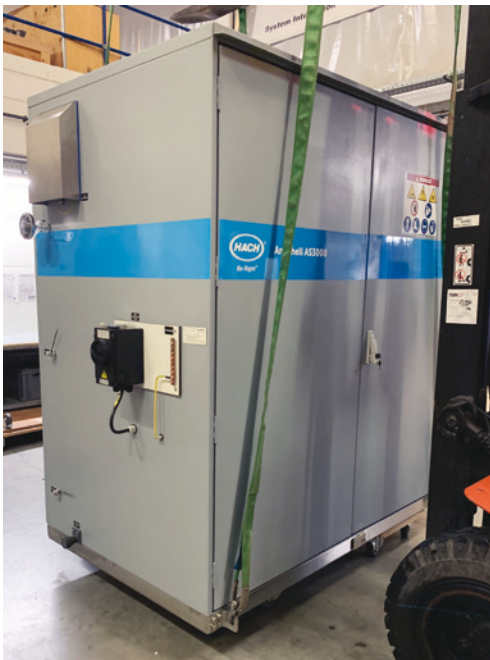
The lifting brackets on the base frame can be twisted by 90° for mounting at the final destination.
