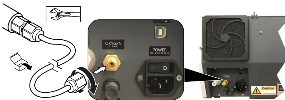
Figure 6 Connect to carrier gas
