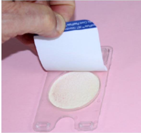
Figure 2: Step 2 of Hach Peel Plate Method
