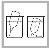
**3.** Collect at least 40 mL of sample in a 50-mL beaker. Fill a NitraVer 5 Nitrate AccuVac Ampul with sample. Place a stopper over the tip of the ampul.
