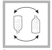
**4.** Press the soft key under *START TIMER*. A one-minute reaction period will begin. Invert the ampul repeatedly until the timer beeps. Wipe off any liquid or fingerprints.
