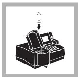
**10.** Place the AccuVac ampul into the cell holder. Close the light shield. Results in mg/L nitrate expressed as nitrogen (NO<sub>3</sub>-N) will be displayed.
