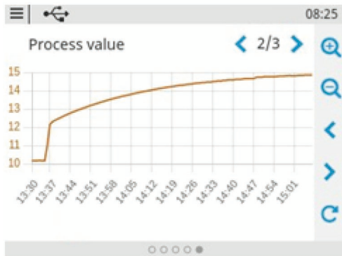
Figure 1 PID tuning with a setpoint at 15
