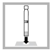
7. Insert the vial into the cell holder. DR1900: Go to LCK/TNTplus methods. Select the test, push **READ**.
