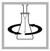
11. Put the delivery tube point fully into the solution and swirl the flask. Turn the knob on the Digital Titrator to add titrant to the solution. Continue to swirl the flask and add titrant until the color changes to a permanent blue color. Record the number of digits on the counter.
