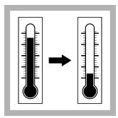
**9.** When the timer expires, set the reactor power to off. Let the temperature decrease for about 20 minutes to 120 °C (248 °F) or less.
