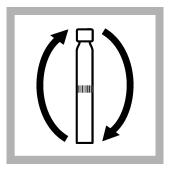
Hold the vial by the cap, over a sink. Invert gently several times to mix. The vial gets very hot during mixing.
