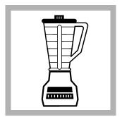
2. Measure 100 mL of sample in a blender. Blend for 30 seconds or until homogenized. If the sample does not have suspended solids, ignore this step.
