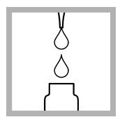
**5.** Use a pipet to add 2.0 mL of sample to the test vial.
