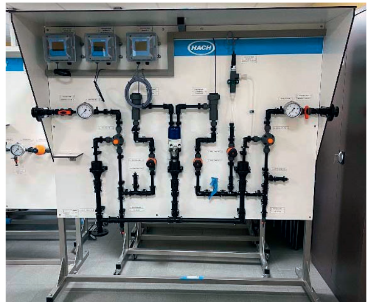
Anarack analyser rack for pH, conductivity and temperature sensors
