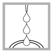
**6.** Add 0.5 mL of 0.3% PAN Indicator Solution to each cell. Use the plastic dropper supplied.
