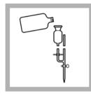
1. Fill the 5-mL automatic buret to the zero mark with 0.00564 N Phenylarsine Oxide (PAO) Solution.
