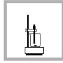
5. Place the beaker of prepared sample on the TitraStir titration stand and turn on the stirring motor. Put the tip of the probe fully into the prepared sample. The platinum wires must be submerged.
