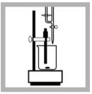
8. Continue dispensing slowly. Near the end point of the titration, write down the value on the display and the corresponding total volume of titrant that was added. Read the volume to the nearest 0.01 mL. Add a small amount of titrant and wait several seconds for a stable value. Write down the value.
