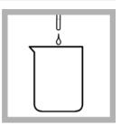
**4.** Add 1.0 mL of pH 4 Acetate Buffer Solution to make the prepared sample.
