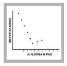
**9.** Continue the titration by recording at least three points on the downward sloping curve and at least three points after the end point has been reached. The value on the display will not change significantly after the end point.
