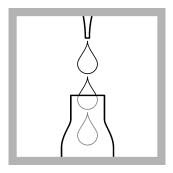
2. Pipet 4.0 mL distillate into the vial.
