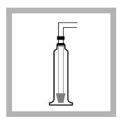
1. Use MEBAK or ASBC analysis methods to distill 100 g of uncarbonated beer to 25 mL of sample distillate. Use the sample distillate in the test procedure.
