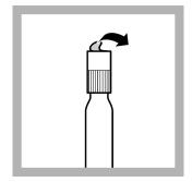
**8.** Carefully remove the foil from the screwed-on DosiCap Zip.
