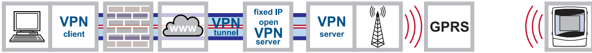
Figure 23 GPRS connection via fixed IP service and VPN server of the mobile network operator
