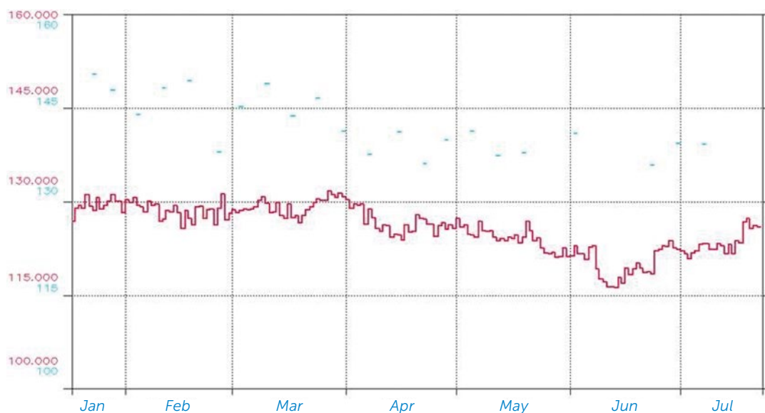
Data trend of the online analyser (red) and spot lab measurements (to be divided by 1.22)
