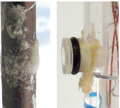
Innocuous crystallisation on storage cap, electrode shaft or refill opening
