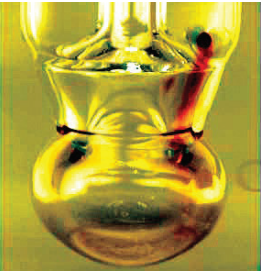
Correctly functioning ceramic diaphragm, effluence of electrolytes (red liquid)
