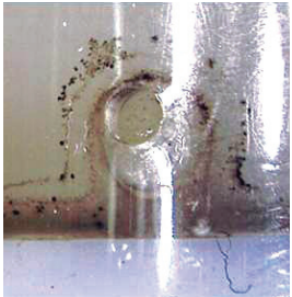
Contaminated reference junction
