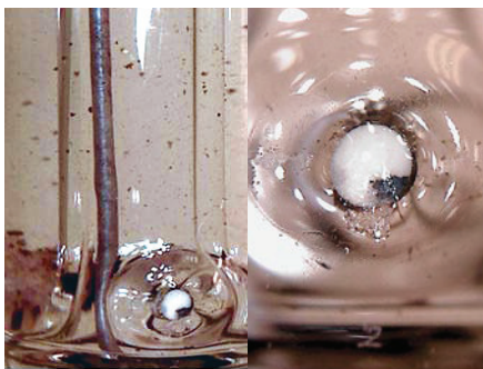
Ceramic diaphragm after treatment with KS410 solution
