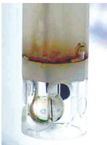
Contaminated (left) and clean (right) gel electrolyte
