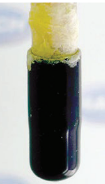
Innocuous crystallisation on storage cap, electrode shaft or refill opening
