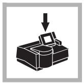
**15.** Read the mg/L phosphate from the display. Multiply this value by the appropriate multiplier in *Table 2* to obtain the actual concentration of phosphates in the sample.
