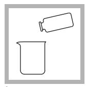
**9.** Pour off about 15 mL of sample into a 50-mL beaker so that 10 mL remains in the 1-inch sample cell. This is the prepared sample.
