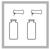
**10.** Add the contents of one PhosVer 3 Phosphate Reagent Powder Pillow to the blank and prepared sample. Swirl immediately to mix.
