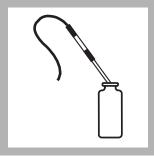
**6.** Insert the ultraviolet (UV) lamp into the sample cell.
