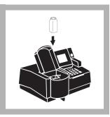
**14.** Place the prepared sample in the cell holder. Close the light shield.
