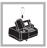
**12.** When the timer beeps, place the blank (undigested sample) into the cell holder. Close the light shield.
