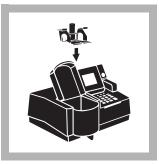
**6.** Insert the Test 'N Tube Adapter into the sample cell module by sliding it under the thumb screw and into the alignment grooves. Fasten with the thumb screw.
