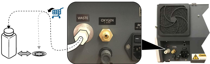
Figure 6 Connect the waste tubing
