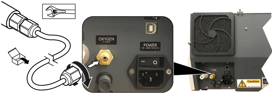
Figure 5 Connect to carrier gas
