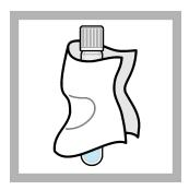
**13.** When the timer ends, clean the external surface of the sample vial with a no-lint cloth.
