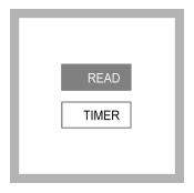
17. Select **READ**. The results show in ppb ( $\mu$ g/L). If the sample temperature is higher or lower than 20  $\pm$  3 °C (68  $\pm$  5 °F), refer to Temperature correction to calculate the actual reading.
