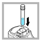
**14.** Put the sample vial in the vial adapter.
