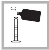
**5.** Add 30 mL of chloroform to a 50-mL mixing graduated cylinder. Add the contents of one DithiVer Metals Reagent Powder Pillow. Stopper the cylinder. Invert several times to mix (this is the DithiVer solution).
