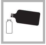
**11.** Fill a dry 25-mL sample cell with chloroform (the blank). Stopper.
