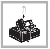
14. Place the prepared sample into the cell holder. Close the light shield. Results in μg/L cadmium (or chosen units) will be displayed.
