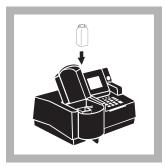
**12.** Place the blank into the cell holder. Close the light shield.
