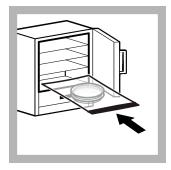
**11.** Incubate the inverted petri dish at 35 (± 0.5) °C (95 (± 0.9) °F) for 48 hours.
