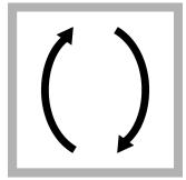
3. Invert the sample or the diluted sample for 30 seconds (25 times) to make sure that the sample is mixed well.
