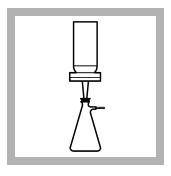
**5.** Apply the vacuum until the funnel is empty. Stop the vacuum.
