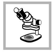
12. Remove the petri dish from the incubator. Use a 10 to 15x microscope to count the number of bacteria colonies on the membrane filter that have a clear to cream color. Refer to Interpret and report the HPC results on page 4.
