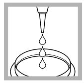
1. Open one m-TSB-USP broth ampule. Lift the lid of a petri dish and carefully pour the contents equally on the absorbent pad.
