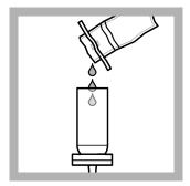
**4.** Pour or use a pipet to add the sample into the funnel. If the volume is less than 20 mL, add 10 mL of sterile buffered dilution water to the funnel.
