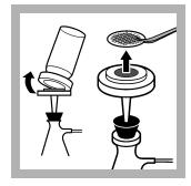
7. Stop the vacuum when the funnel is empty. Remove the funnel from the filter assembly. Use sterile forceps to lift the membrane filter.
