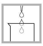
**3.** Add 1 mL of 1.0 N Hydrochloric Acid Standard Solution to the beaker.
