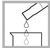
2. Prepare the sample: Collect 50 mL of sample in a 100-mL beaker.
