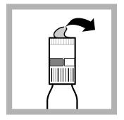
Carefully remove the lid from the DosiCap<sup>™</sup> Zip cap. Remove the cap from the test vial.
