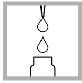
2. Use a pipet to add 5.0 mL mL of sample to the test vial. Immediately continue to the next step.
