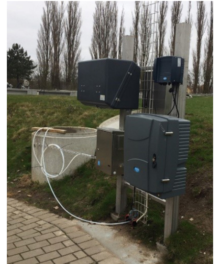
Figure 2: Hach Amtax sc Ammonium Analyzer, Nitratax sc Nitrate Sensor, and SC1000 Controller Probe Module.
