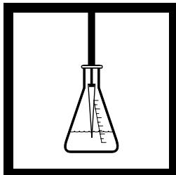
**7.** Use the pipettor to dispense two volumes (200  $\mu$ L) of bleach sample below the solution level in the flask.
