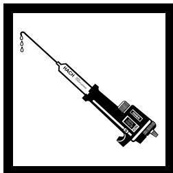
2. Flush the delivery tube by turning the delivery knob to eject a few drops of titrant. Reset the counter to zero and wipe off the tip.
