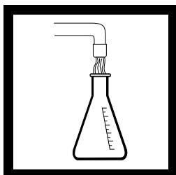
3. Fill the erlenmeyer flask to about the 75-mL mark with deionized or tap water.
