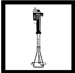
9. Place the delivery tube tip into the solution and swirl the flask while titrating with the thiosulfate titrant until the solution is light yellow.
