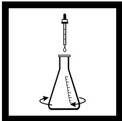
10. Add one dropperful of starch indicator solution to the flask and swirl to mix. A dark blue or green color will develop.
