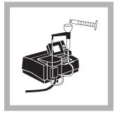
11. When the timer beeps, introduce the contents of the cylinder into the Flow-Thru Cell or Sipper Cell.
