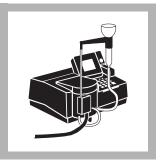
14. When the timer beeps, the result in  $\mu g/L$  (or chosen units) chlorine will be displayed.
