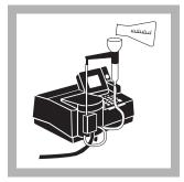
**4.** Pour at least 50 mL of sample into the Flow-Thru or Sipper Cell.
