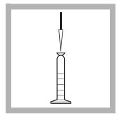
**8.** Using a TenSette Pipet and clean tip, transfer 1.0 mL of buffer from the ampule to a clean, treated 50-mL graduated mixing cylinder.
