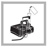
**13.** Flush the Flow-Thru or Sipper Cell with at least 50 mL of deionized water immediately after use.
