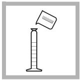
7. Fill the cylinder to the 50-mL mark with the dechlorinated water from Step 3. Cap and invert twice to mix. Save the remaining water for Step 9.
