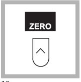
**10.** When the flow stops, press the soft key under **ZERO**.
