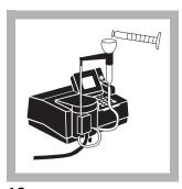
**13.** Introduce the contents of the graduated mixing cylinder into the Flow-Thru or Sipper Cell.
