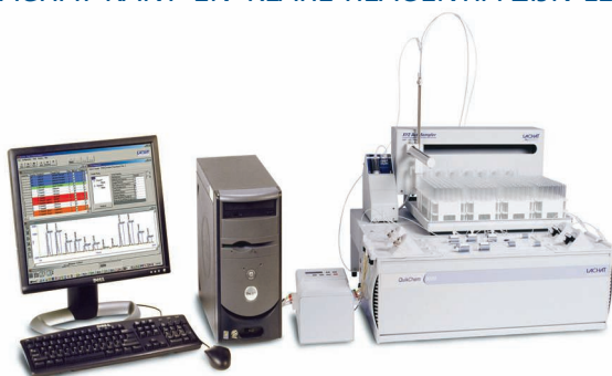
QuikChem 8500 Flow Injection Analysis System
