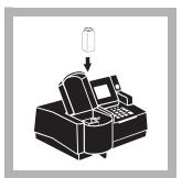
10. Within eight minutes after the timer beeps, place the prepared sample into the cell holder. Close the light shield. The result in mg/L Mn (or chosen units) will be displayed.
