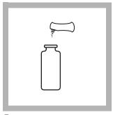
**5.** Add the contents of one Sodium Periodate Powder Pillow to the sample cell (the prepared sample). Swirl to mix.
