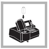
**8.** When the timer beeps, place the blank into the cell holder. Close the light shield.
