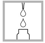
**8.** Use a pipet to add 0.4 mL of Solution B to the test vial.
