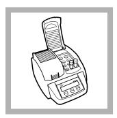
**5.** Insert the vial in the preheated DRB200 reactor. Close the lid.
