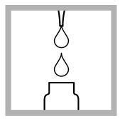
**2.** Use a pipet to add 0.4 mL of Solution A to the test vial.
