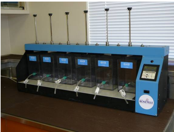
Figure 39: Wagner™ Jar with Phipps Bird Multiple Stirrer
