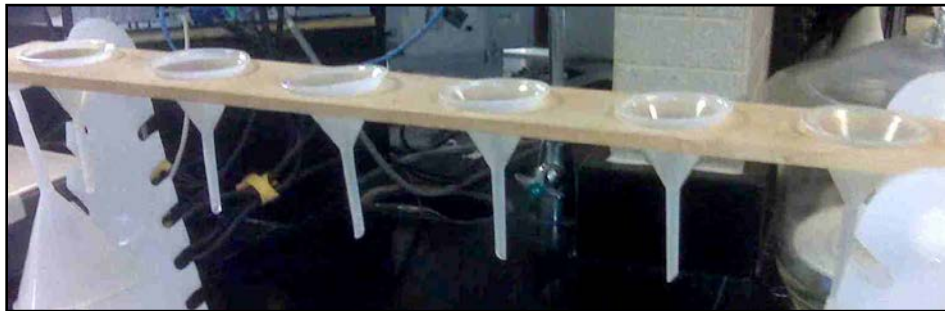
Figure 40: Six-place assembly for filtering samples after a jar test
