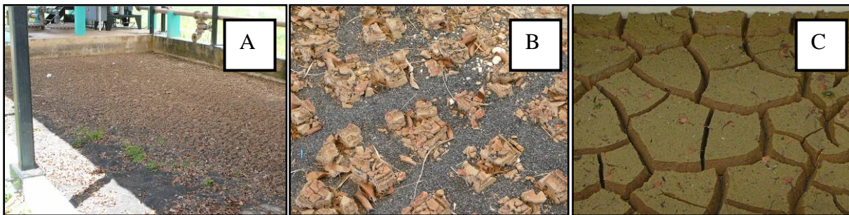
Figure 28: Anthracite Loss Due To Backwash
