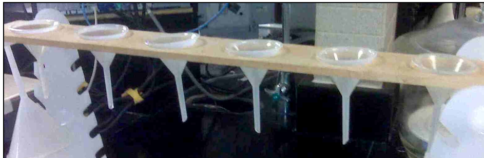
Figure 21: Six-place assembly for filtering samples after a jar test. Photo by author.
