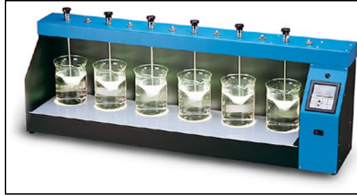
Figure 18: Jar test apparatus Phipps Bird 6-Place Programmable Multiple Stirrer with 1-liter round glass beakers. Hach Company stock photo
