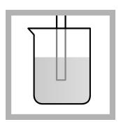
**19.** Measure the pH of the remaining sample from the analyzed bottle to examine the pH changes that can occur in waters with low alkalinity.
