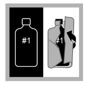
**13.** Put the sample bottle in a dark location or wrap with foil.
