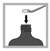
**5.** Use tweezers or tongs to put a stir bar magnet into each bottle. Do not touch the stir bar.
