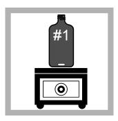
**6.** Put Bottle #1 on the stir plate. Set a low stir speed. A small vortex will show on the surface of the liquid.
