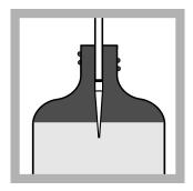
8. Use a TenSette Pipet to add 0.2 mL of the chlorine solution to Bottle #1 while stirring. Put the end of the pipet tip under the water to dispense the chlorine. To prevent highly localized areas of chlorine concentration is mandatory to stir the sample while the chlorine is added.
