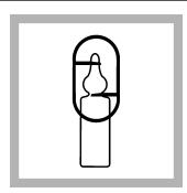
**7.** Use the ampule breaker to open a Chlorine Dosing Solution Ampule.
