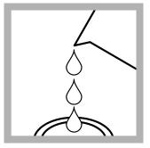
**4.** Fill each 118-mL bottle with approximately 100 mL of the collected sample. If constant pH is required, add the pH buffer to the sample before the bottles are filled.
