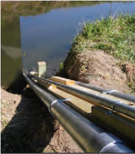
Photo 4: Example pipe deployment of optical nitrate sensor into environmental waters from the bank of a river. (Credit: U.S. Geological Survey report, 2013)
