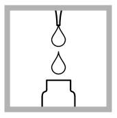
2. Prepare the blank: Use a pipet to add 11 mL of the sample to an empty 16-mm vial.
