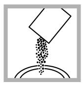
**6. Prepare the sample:** Add the contents of one DPD Total Chlorine Powder Pillow for 25-mL to a clean, empty vial.
