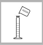
**10.** Avoiding extra agitation, carefully fill the cylinder to the 50-mL mark with sample. Stopper. Gently invert it twice to mix (the prepared sample).
