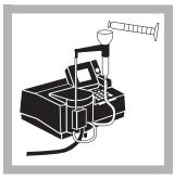
**11.** When the timer beeps, introduce the contents of the cylinder into the Flow-Thru Cell or Sipper Cell.
