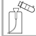
**13.** Insert the plunger into the barrel and slowly push the plunger down with even pressure, until the plunger is fully seated.
