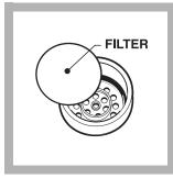
**5.** Install a new 3-micron filter into the cap well. Wet the filter with a few drops of deionized water. Reassemble and hand-tighten the cap onto the plunger.
