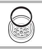
**4.** Unscrew the cap from the OriFlo plunger assembly. Be sure the O-ring is properly seated in the cap.
