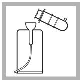
**20.** Introduce the filtered reacted sample from the beaker into the Flow-Thru or Sipper Cell.
