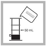
**12.** During the 3-minute reaction period, push the valve button on the OriFlo barrel assembly to the "closed" position. Place the barrel assembly into its stand. Pour approximately 50-mL of the original sample into the barrel.
