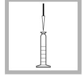
**9.** Using a TenSette Pipet and clean tip, transfer 1.0 mL of indicator from the ampule to the graduated mixing cylinder. Swirl to mix the reagents. Proceed with Step 10 within 1 minute.
