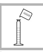
**7.** Fill the cylinder to the 50-mL mark with the dechlorinated water from Step 3. Cap and invert twice to mix. Save the remaining water for Step 9.
