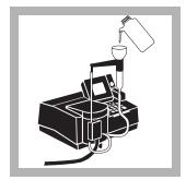
**13.** Flush the Flow-Thru or Sipper Cell with at least 50 mL deionized water immediately after use.
