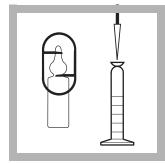
**5.** After the timer beeps, break open 1 ampule of ULR Chlorine Buffer Solution. Using a TenSette Pipet and clean tip, transfer 1.0 mL of buffer from the ampule to a clean 50-mL mixing graduated cylinder.
