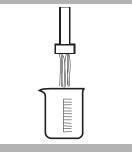
**2.** Collect about 100 mL deionized or tap water in a clean 250-mL beaker.
