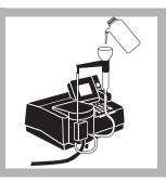
**22.** Flush the Flow-Thru or Sipper Cell with at least 50 mL of deionized water immediately after use.
