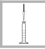
**7.** Using a TenSette Pipet and clean tip, transfer 1.0 mL of buffer from the ampule to a clean, treated 50-mL graduated mixing cylinder.
