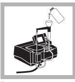
**3.** Install the 1-inch Flow-Thru or Sipper Cell Module in the instrument. Flush it with at least 50 mL of deionized water.
