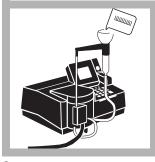
**9.** During the reaction period flush the Flow-Thru or Sipper Cell with the remainder of the original dechlorinated water from Step 7.
