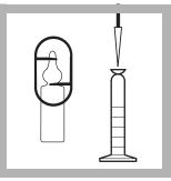
**6.** Break open 1 ampule of DPD Indicator Solution for Ultra Low-Range Chlorine. Using a TenSette Pipet and clean tip, transfer 1.0 mL of indicator from the ampule to the cylinder. Swirl to mix the reagents. Proceed with Step 7 within 1 minute.
