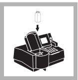
10. Place the prepared sample into the cell holder. Close the light shield. Results in mg/L chloride (or chosen units) will be displayed.
