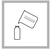
**3.** Fill a sample cell with 25 mL of sample (the prepared sample).
