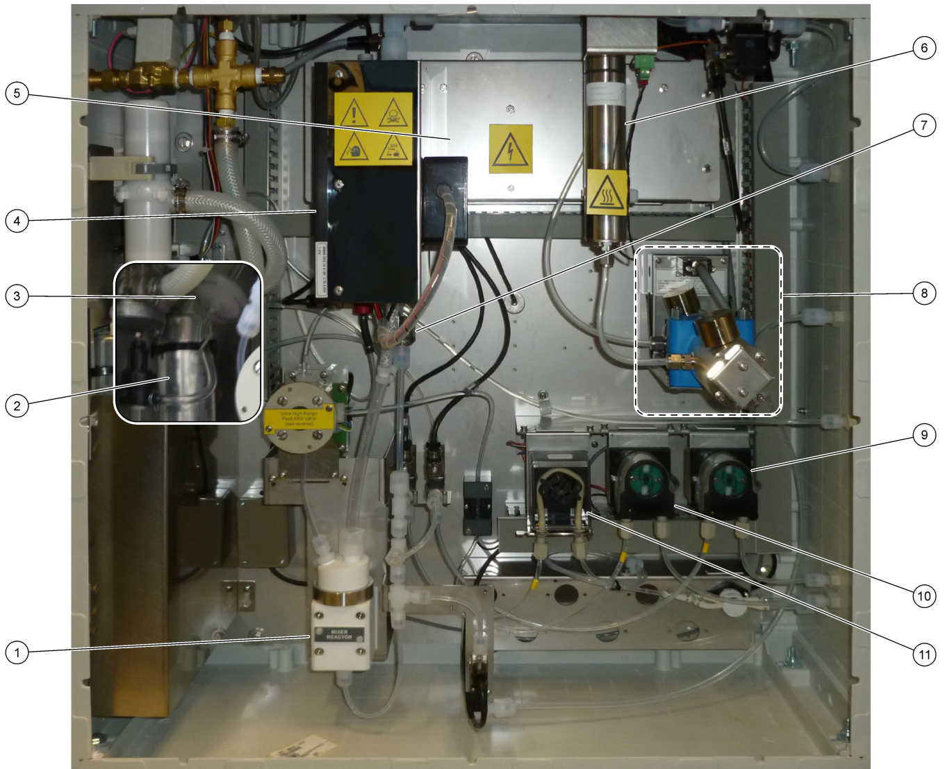
Figure 9 Analysis enclosure—Pumps and components
