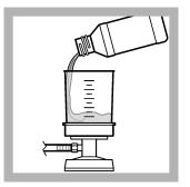
**4.** Rinse the funnel walls 3 times with 20 to 30 mL of sterile buffered dilution water. Use the syringe to pull the water through the filter after each rinse.
