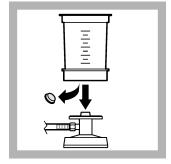
**1.** Remove the plug from the filter assembly. Push the filter assembly on the manifold.
