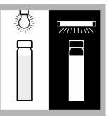
10. Apply UV light to the incubated sample that contains MUG broth with a long-wave UV lamp. Examine the tubes in a dark area. Look at the tube 90° from the UV light. Compare the fluorescence of the sample tubes to a tube that contains a known E. coli positive confirmation. If the sample fluoresces, E. coli bacteria are in the sample. If the sample does not fluoresce, the test is negative for E. coli.
