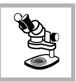
**10.** Remove the petri dish from the incubator. Use an illuminated magnifier or 10x to 15x microscope to count the number of red or magenta colonies.
