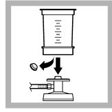
**1.** Remove the plug from the filter assembly. Push the filter assembly on the manifold. Remove the petri dish from the top of the filter assembly.
