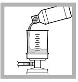
**3.** Pour 100 mL of the diluted sample into the funnel. Pull the plunger on the syringe to pull the sample through the filter.
