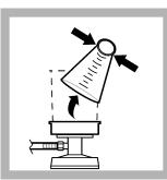
**6.** Squeeze the top of the funnel and remove the funnel from the filter assembly.
