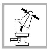
**5.** Squeeze the top of the funnel and remove the funnel from the filter assembly.
