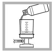
**5.** Rinse the funnel walls 3 times with 20 to 30 mL of sterile buffered dilution water. Use the syringe to pull the water through the filter after each rinse.
