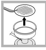
7. Use sterile forceps to lift the membrane filter from the base of the filter assembly.
