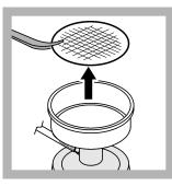
**6.** Use sterile forceps to lift the membrane filter from the base of the filter assembly.
