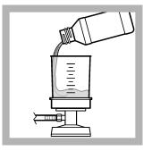
**4.** Pour 100 mL of the diluted sample into the funnel. Pull the plunger on the syringe to pull the sample through the filter.
