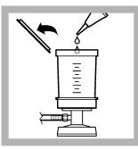
2. Open one m-FC broth ampule. Lift the cover of the filter assembly and pour the contents equally on the absorbent pad in the petri dish. Remove the petri dish from the filter assembly.
