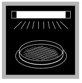
5. Remove the lid from the petri dish. Apply UV light to the colonies in a dark area. If the colonies fluoresce, *E. coli* bacteria are in the sample. If the colonies do not fluoresce, the test is negative for *E. coli*.
