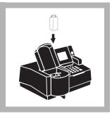
**8.** Gently invert the prepared sample several times. Immediately place it into the cell holder. Close the light shield. Results in FAU turbidity will be displayed.
