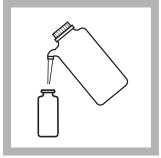
**3.** Use a set of matched sample cells. Fill one of the clean stoppered sample cells to the 10-mL mark with deionized water (the blank). Stopper.
