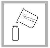
**4.** Rinse the other matched sample cell with sample. Then fill the sample cell to the 10-mL mark with sample. Stopper (this is the prepared sample).
