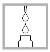
2. Use a pipet to add 0.2 mL of sample to the test vial. Immediately continue to the next step.
