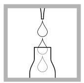
2. Carefully pipet 0.2 mL of solution A.
