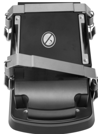
Illustration 10: Placing the clamp straps
