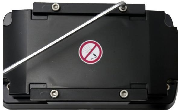
Illustration 5: Loosen screws on MARWIS-UMB housing
