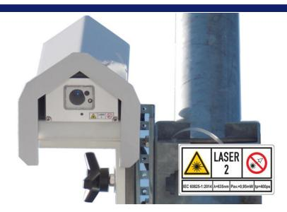
The laser-based snow depth sensor Lufft SHM31 stands for millimeteraccurate snow level detection over long distances in all weather conditions without any maintenance, due to opto-electronic/laser based rangefinder technology.
