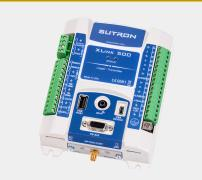
A multi-sensor input logger, for digital and analog sensors, with data transmission via Iridium or Cellular. Includes custom Python Scripting and compatible with the easy-to-use LinkComm GUI interface via WiFi or directly with any smart device.
