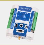
A multi-sensor input logger, for digital and analog sensors, with data transmission via Iridium or Cellular. Includes custom Python Scripting and compatible with the easy-to-use LinkComm GUI interface via WiFi or directly with any smart device.
