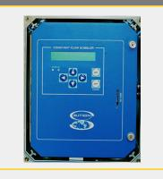
Self-contained, precision device to measure water level and temperature. Equipped with auto-purge capabilities to prevent or clear orifice line blockages.
