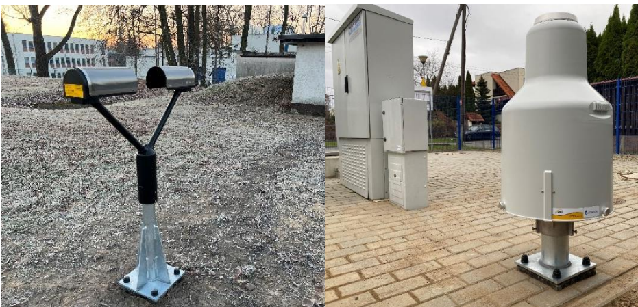
OTT Parsivel Disdrometer (left). OTT Pluvio 2 L and a standing cabinet (right).
